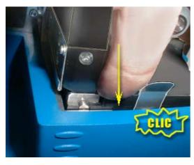
• Push down the card carrier with your finger until it is locked down
