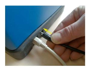
• Connect the JACK connector to the printer
