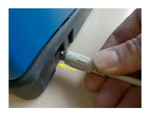
Only use the serial cable supplied with the printer
