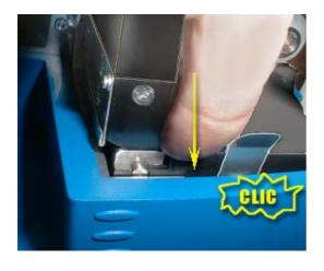
• Push down the card carrier with your finger until it is locked down
