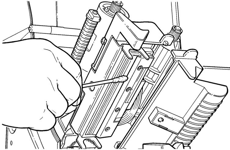
8. Rub the cotton swab across the supply sensor and remove any build-up.
