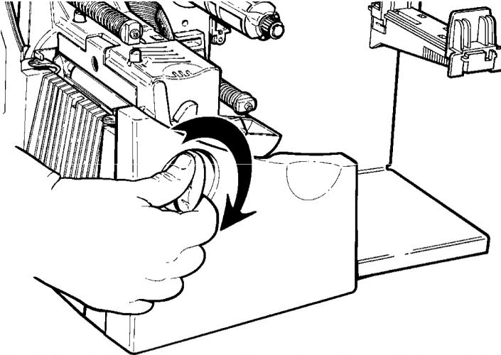
3. Lift printhead assembly using the printhead tab until the assembly locks into place.
