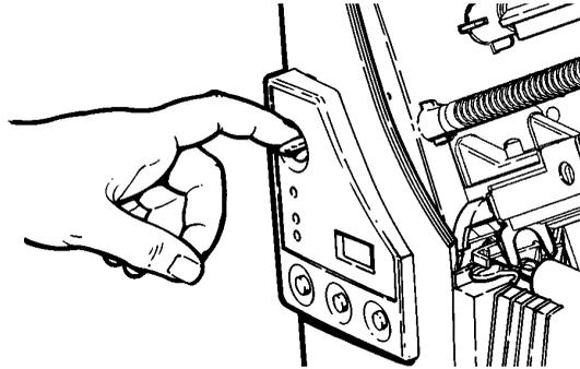
14. Close the printhead by pressing down on the thumb well until you hear it click into place. Close the cover.
