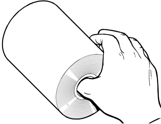
7. Slide the ribbon onto the back reel as far as it will go. The ribbon roll only fits on the reel one way. Carefully unwind a few inches of ribbon from the bottom of the roll.
