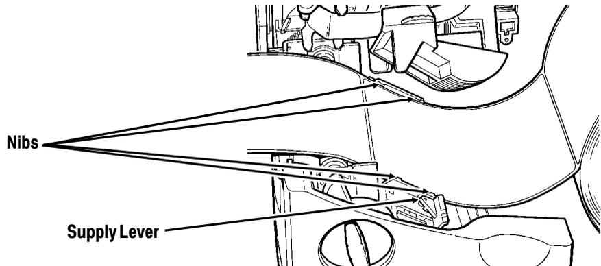
8. Adjust the supply guides so they touch the supply. Push up on the supply lever to lock the supply guides into place.
