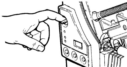
10. Close the printhead by pressing down on the thumb well until you hear it click into place.
