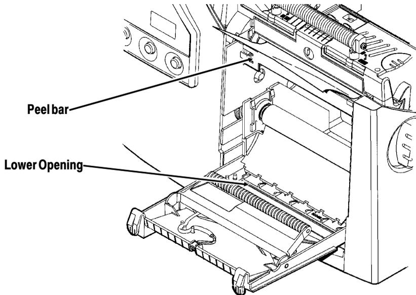
14. Feed the backing paper through the lower opening of the exit cover. Pull down on the backing paper to remove any slack. Close the exit cover.
