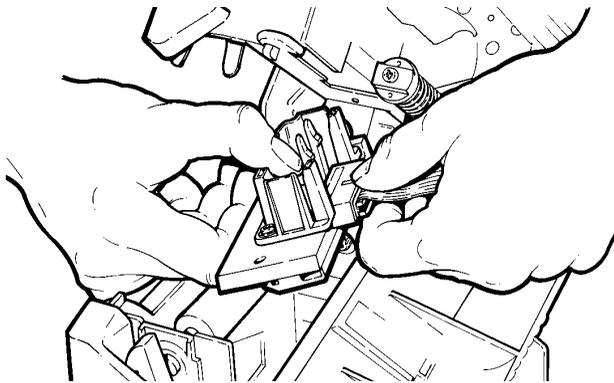
7. Carefully plug the cable into the new printhead.
