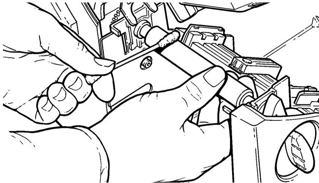
6. Rub the cotton swab across the peel bar and remove any build-up. The peel bar is only available on the 9830 printer.
