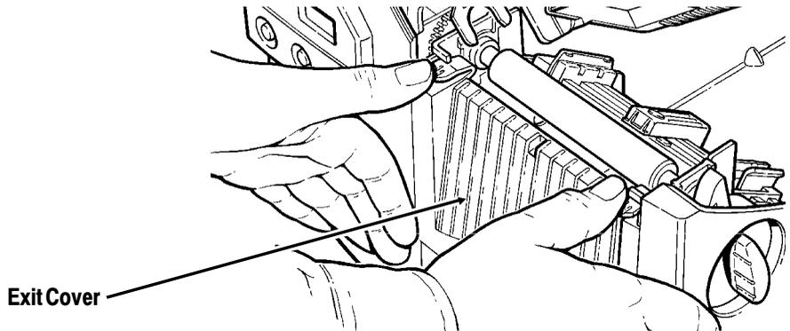
13. Feed the backing paper over the peel bar.
