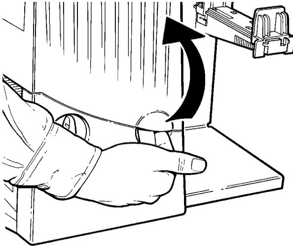
2. Unlock the printhead by turning the retaining latch.
