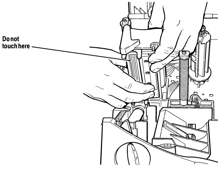
Make sure the printhead cable does not touch the ribbon roll.
