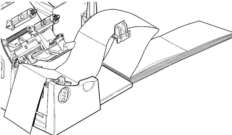
7. Adjust the supply guides so they touch the supply. Push up on the supply lever to lock the supply guides into place.
