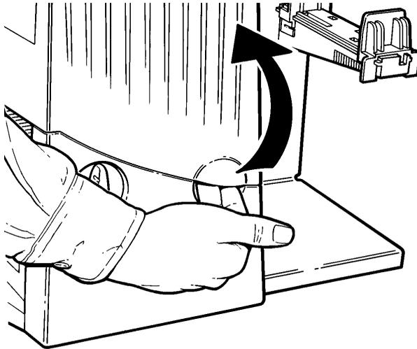
2. Unlock the printhead by turning the retaining latch.
