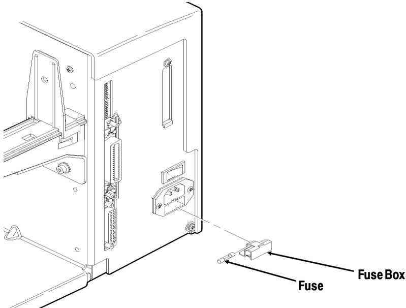
2. Use a screwdriver to pry open the fuse box in the back of the printer.
