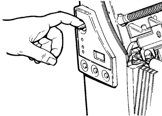
10. Close the printhead by pressing down on the thumb well until you hear it click into place.
