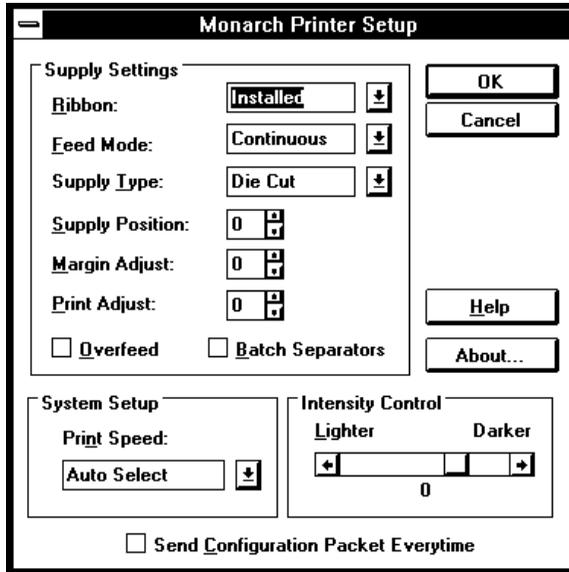
You can change any of the following setup options: Ribbon, Feed mode, Supply Type, Supply/Print/Margin positions, Print Speed, and Print Contrast. You can also enable Overfeed or Batch Separators.
