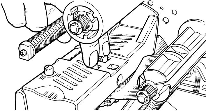
5. Lift the printhead assembly using the printhead tab and push back until the printhead assembly clicks into place.
