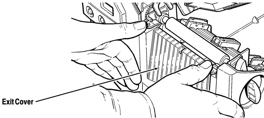
5. Moisten a cotton swab with isopropyl alcohol. Turn the platen roller with your finger and run the cotton swab across it. Make sure the platen roller is clean all the way around.
