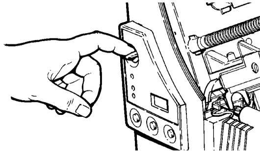
9. Close the printhead by pressing down on the thumb well until you hear it click into place.
