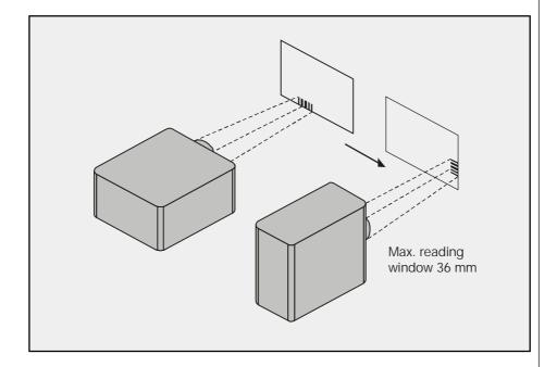
The recording time of code cameras is extremely short, which means that it is possible to record both stationary and fast-moving coding. Because the code camera records the code as a whole, orientation in machine or traverse direction is possible.
