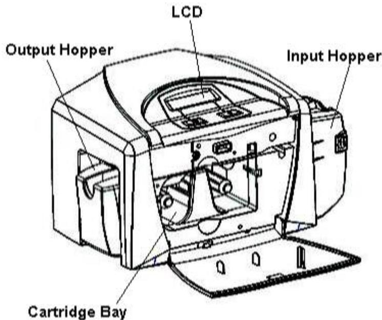
**Reviewing the DTC400/DTC300/DTC300M Sequence of Operations (continued)**
