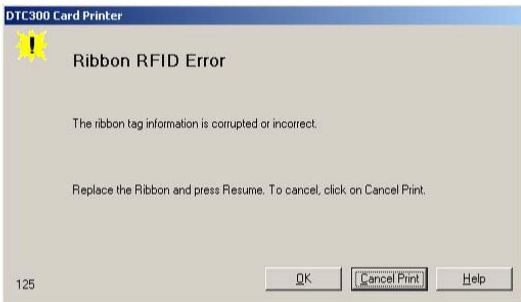
**Resolving a Ribbon RFID Error (Ribbon RFID Antenna is Corrupted)
