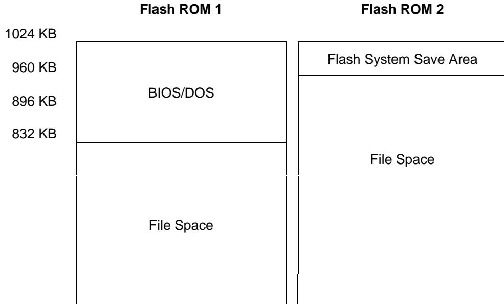
The printer uses 1K to 5K of the file space for the file access table. The table's size depends on the number of files in the disk image and the space they use.
