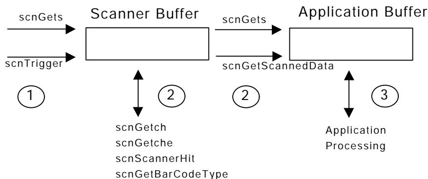
The scanner contains a buffer to hold the data from a scan. The application should contain a buffer of its own if it needs to save the data before scanning again. Processing works as follows:
