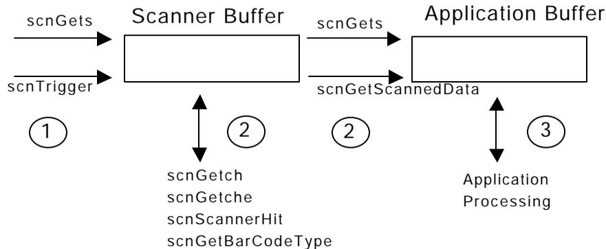
The scanner contains a buffer to hold the data from a scan. The application should contain a buffer of its own if it needs to save the data before scanning again. Processing works as follows:
